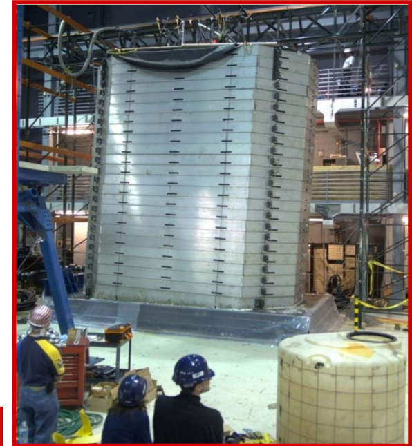
Large Scale Liquefaction Tests (U. Buffalo)
